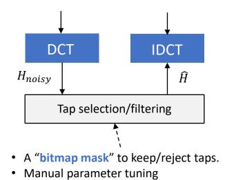
Al-based tap selection/filtering enabling weighting instead of selection
